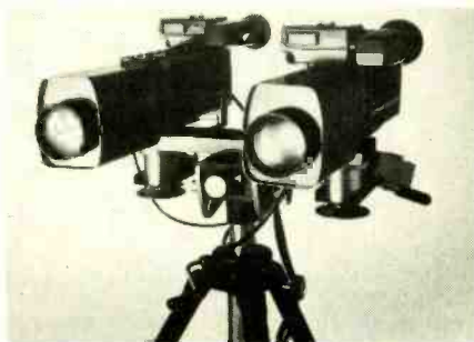
FIG. 2—TWO VIDEO CAMERAS, one for the right-eye image, and one for the left-eye image, are required for 3-D television.
