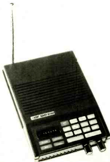
FIG. 6—THIS COMPACT SCANNER, for the Fox BMP 10/60 from ComRadar Corporation, features 60 pre-programmed frequencies.
